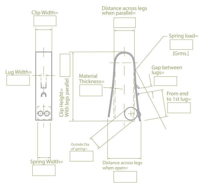
For the purpose of quotation (prior to sending any damaged / broken spring clips through to us), please advise the following details to enable us to select the most appropriate replacement spring coil:
